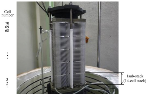
Fig. 15. Present 70-cell stack (2.5 kW class stack).
